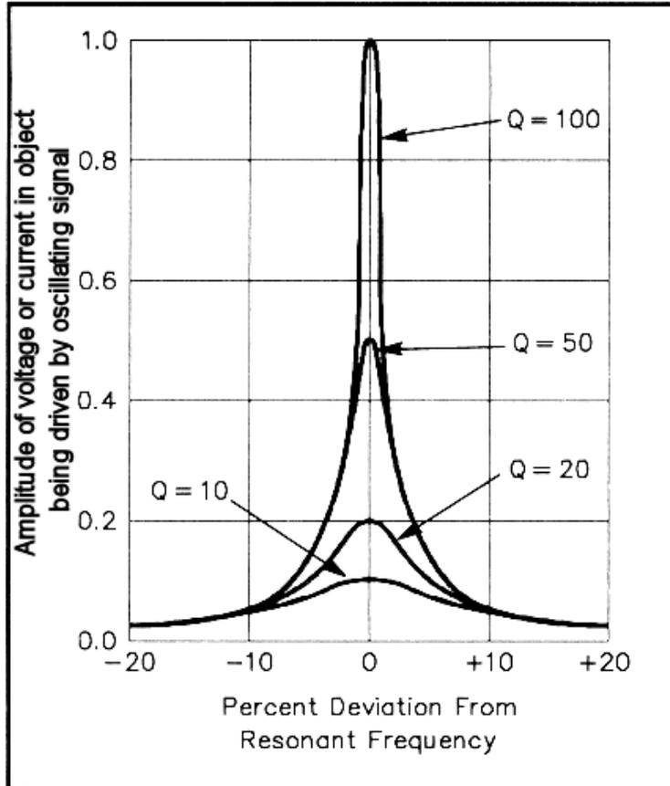
The illustration above shows how low Q factor makes the response curve much flatter, meaning a resonance point is much less unique.
